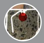
Patented Dincel barbs and cement slurry ensures that snap joint is waterproof
