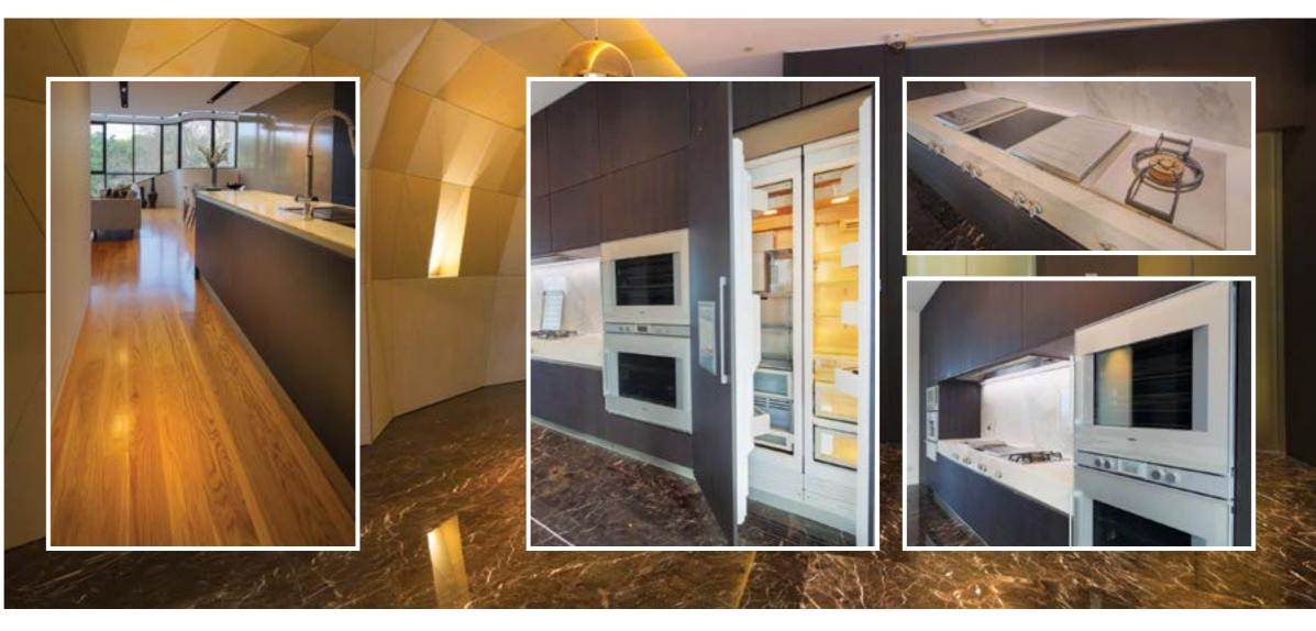
The flooring timber was then installed using glue and secret nails, sanded and polished and finished with three coats of polyurethane varnish. The challenges began with the tight timeframe of only six weeks for the entire scope, which Danzaco achieved through using three teams, working concurrently and each delivering one part of the job – battens, flooring, and finishing.
