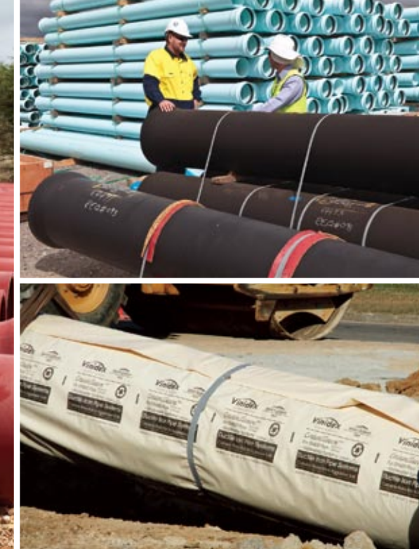
Main: Boulderstone's with 600DN Sewer Ductile Iron Pipe. Top: Vinidex & Boulderstone staff with PE pipe and Vinidex Supermain® PVC-O. Top 2nd: Construction of pipe system. Bottom: Vinidex polyethylene pipe.
