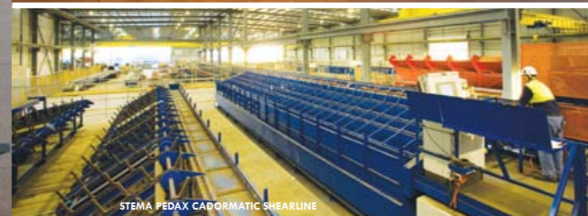
VIEW OF PINKENBA FACTORY SHOWING BOTH DOWN SHOP AND ACROSS SHOP BAR PROCESSING ARRIVING AT SINGLE LOAD ASSEMBLY POINT
