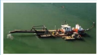
Maritime Constructions was contracted to dredge the top layers of fill, silt and St Kilda clay up to a depth of 5.5m LAT, within the Ship Lift and Main Wharf areas, using a cutter suction dredge. The 5.5m cut-off level represented the bottom of the St Kilda clay geological layer which was to be pumped into a settling pond.
