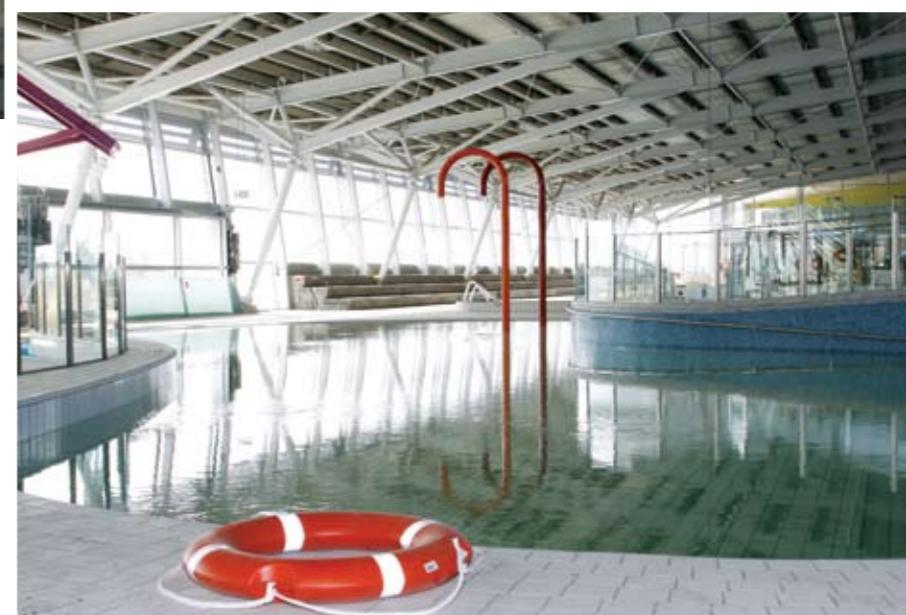
The 51.5m pool and boom are designed to meet FINA requirements for competition length and lane widths and the pool has been fitted out for both 50m and 25m short course events. The boom is normally 'parked' at the deep end of the pool to form an end wall for a 25m short course, or divide the pool, into two. With the boom in a central position, half can be used as a warm up pool for 25m events.
