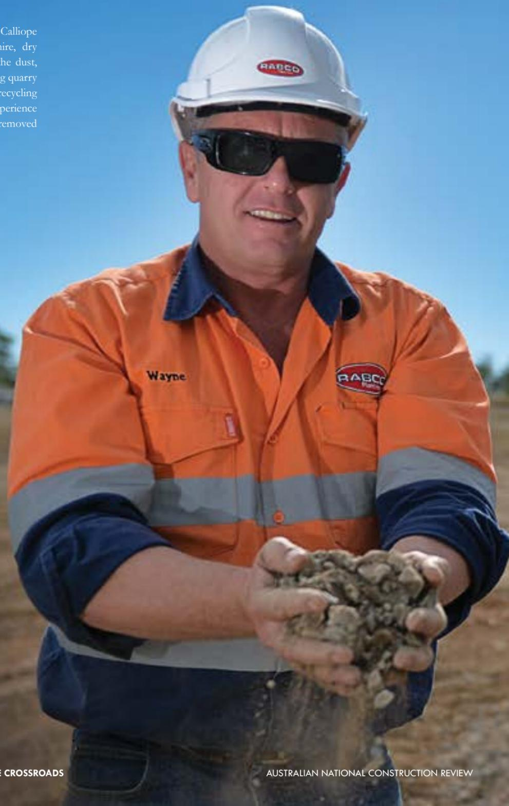
**Right in hands :** The final product produced after Rabco Plant Hire recycled the concrete from the Cross Road Servo. It has been turned into a quality Road Base material.
