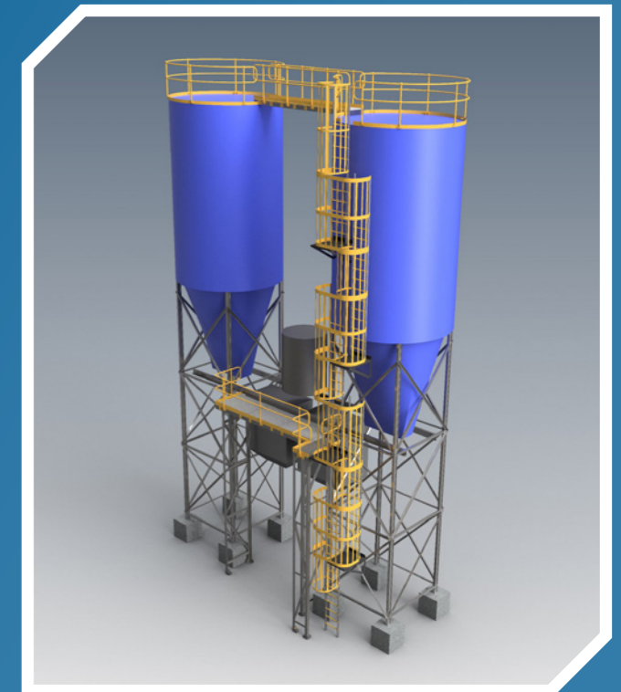
Boral Taree batching plant 3D modelling silo access.
