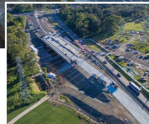
The \$38.8M Telegraph Road upgrade – Stage 2, has been designed to improve safety, travel times, facilities for pedestrians and cyclists, and reduce congestion. The development saw the road widened to incorporate a four-lane median divided carriageway, removal of the existing roundabout to allow for a new signalised intersection, as well as parking areas, shared pathways and dedicated turning bays, and a four-lane three span bridge.
